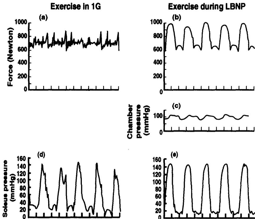
**Figure 3:** Representative recordings during exercise-1G and exercise-LBNP. a & b) Comparison of reaction force waveforms during upright exercise in 1G and supine exercise during 100 mmHg LBNP; c) LBNP chamber pressure fluctuations created by leg exercise-induced movement of the subject; d & e) soleus pressure during exercise-1G and exercise-LBNP.<sup>12</sup>
