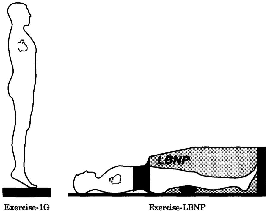
**Figure 2:** Exercise in upright posture against normal gravity (without LBNP) was compared to that during similar exercise in supine posture within the LBNP chamber.
